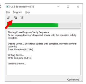
After the firmware has been successfully updated, this is confirmed by the program: "Erase/Program/Verify sequence completed successfully".
