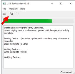
After the firmware has been successfully updated, this is confirmed by the program: "Erase/Program/Verify sequence completed successfully"
