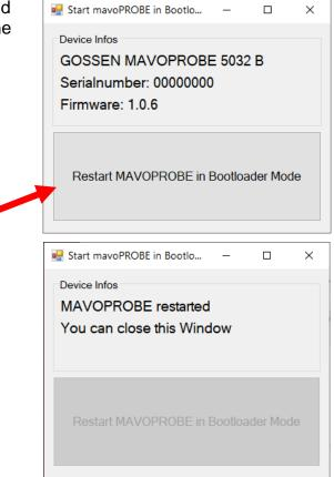
If the device has been found by the software, a message appears: "Device Attached".
