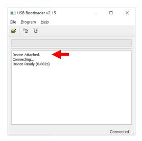
Load the downloaded software by clicking the button. After the firmware file has been successfully loaded, a message appears in the program's main window: "Opened: MavoProbe\_Vxxx.hex". This may take a few seconds.
