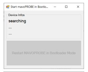
When a MAVOPROBE has been found its Information will be displayed and the Button to restart the MAVOPROBE in bootloader mode is enabled.
