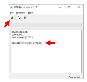
Start the firmware update by clicking the button and wait until the program has completed all installation steps (erasing, writing and verifying). This takes about one minute.
