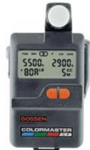
Colormaster 3F - Color temperature meter and filter indicator
